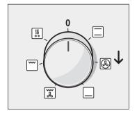
Use the function selector to select the type of heating for the oven.
